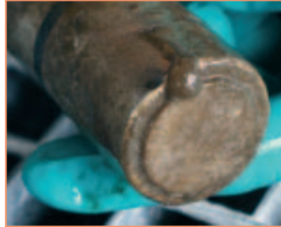
Sensor without ultrasound cleaning system After 16 Days
