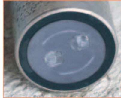
Sensor with ultrasound cleaning system After 16 Days
