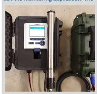
integral data logger will collect data, provide local trending & transfer to pen drive via USB. Option for GSM data transmission. Field replaceable lithium-ion battery packs (external or integrated versions available).
