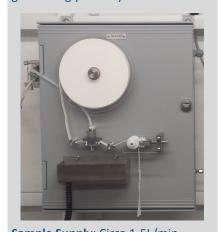
Sample Supply: Circa 1-5L/min Filtrate rate: 10ml/min Sample Temperature: 0-50°C Max Suspended Solids: 250 mg/L
