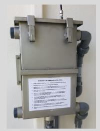
Sample Supply: Circa 1-10L/min Filtrate rate: 10-20ml/min Sample Temperature: 0-45°C Max Suspended Solids: 1,000 mg/L
