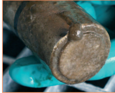
Sensor without ultrasound cleaning system After 16 Days
