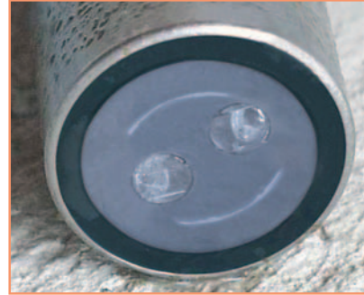
Sensor with ultrasound cleaning system After 16 Days
